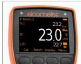
Scan Mode\* stores the average, highest and lowest readings over a test area
