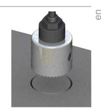
To score coatings thinner than 0.5 mm (20 mils), a sharp knife may be sufficient to carefully score around the dolly once it has been secured in place by adhesive.
