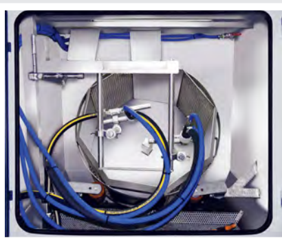
The Aquablast® Tumbler machine featured with 2 stage rinsing, hot and cold, hot rinse not standard. This machine batch processes small parts which are turned in the drum and simultaneously blasted
