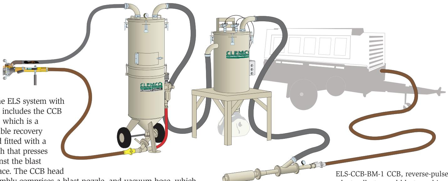
The ELS system with CCB includes the CCB tool, which is a durable recovery head fitted with a brush that presses against the blast surface. The CCB head assembly comprises a blast nozzle, and vacuum hose, which evacuates dust and the rebounding abrasive following its contact with the blast surface. This tough tool contains the abrasive and keeps the surrounding area clean.
