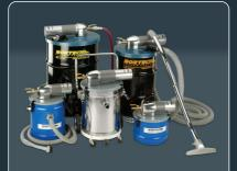
NORTECH VACUUM UNITS Air powered, high productivity vacuums with no electric motors offer safety, durability and the same high level of performance as larger units.
