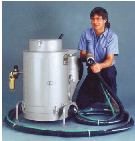
Specialized brushes allow the Comet to clean inside angles, outside angles, smooth, and uneven surfaces.
