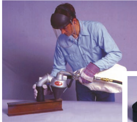
Educt-O-Matic with flat-lip attachment for smooth surfaces.
