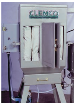
The dust collector houses 12 cotton sateen filter tubes.
