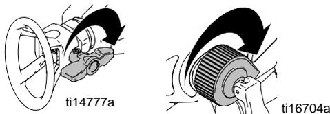
3. Aim sprayer at waste area, disengage trigger lock, and put prime/spray valve DOWN to spray position. Pull trigger to clear clog.
