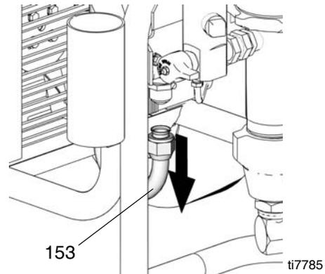
7. Verify drain plug has been replaced. Fill oil reservoir with oil to high mark on dip stick (approximately 3.5 gallons).
