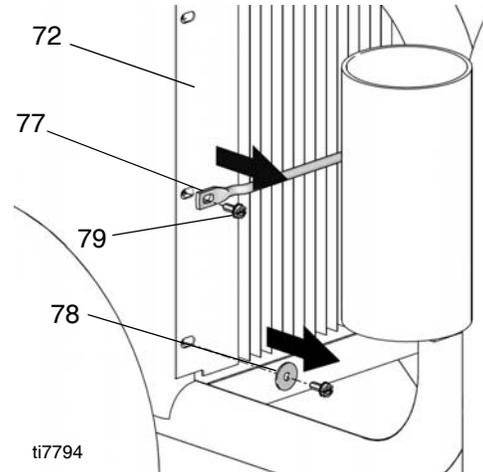
5. Remove coil (72) from sprayer frame.
