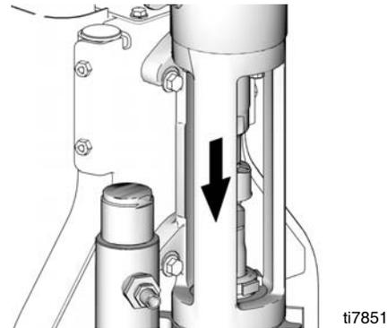
2. Tighten power head bolts (7). Torque bolts to  $400 \pm 10$  in-lb ( $45 \pm 1$  N•m).
