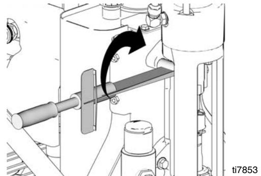
3. Attach hoses (100, 101) to head (75). Torque to  $450 \pm 10$  in-lb ( $50.84$  N•m).
