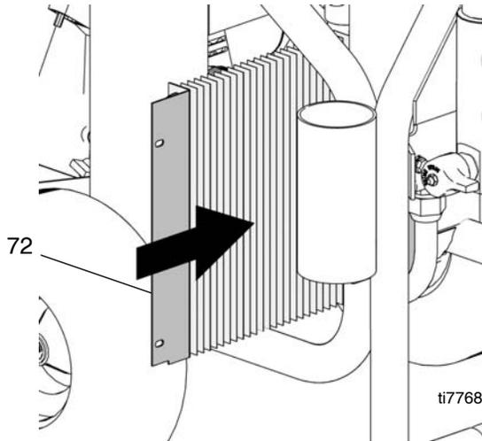
2. Reconnect return line to oil tank and hydraulic line to cooler. Torque to 225 in-lb (25.4 N•m).
