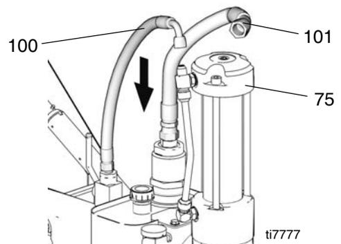
4. To purge air from hydraulic lines, increase pressure enough to start hydraulic motor stroking and allow fluid to circulate for 15 seconds. Turn pressure down. Turn prime valve horizontal (closed).
