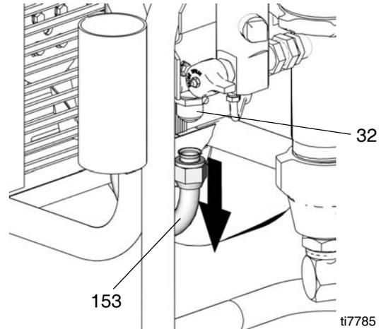
5. Remove and keep suction fitting (32) for use on new reservoir.
