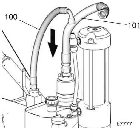
6. Reattach suction hose (153). Torque to  $600 \pm 10$  in-lb ( $68 \pm 1.1$  N•m).
