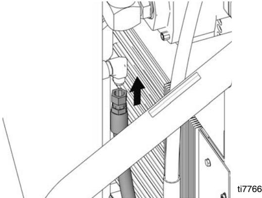
5. Reattach return lines (100, 101). Torque to  $450 \pm 10$  in-lb ( $51 \pm 1.1$  N•m).
