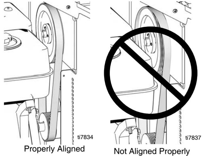
**NOTE:** If belt is not aligned properly, to adjust belt, slowly pull engine recoil while at the same time pushing or pull ing belt to reposition over pulley.
