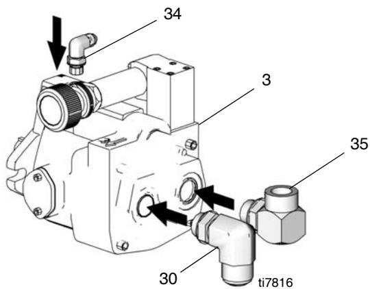
**NOTE:** Fill pump casing with hydraulic oil before installing fitting (34).
