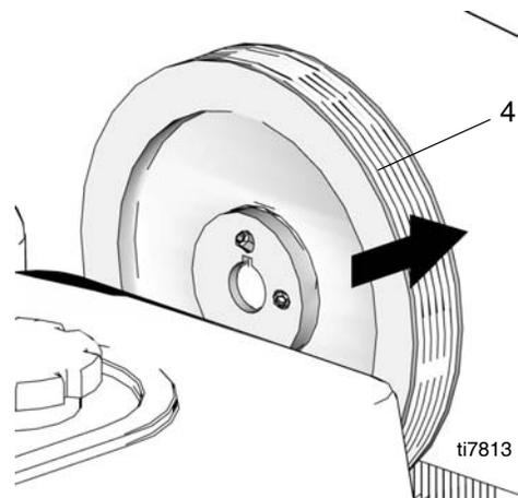
5. Align pulley (4) on shaft. When properly positioned approximately 1/8 inch of shaft (139) will protrude.
