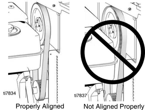
**NOTE:** If belt is not aligned properly, to adjust belt, slowly pull engine recoil while at the same time pushing or pulling belt to reposition over pulley.
