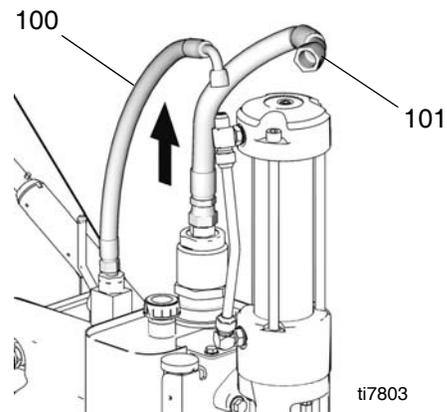
7. Remove cooler line from reservoir (64).
