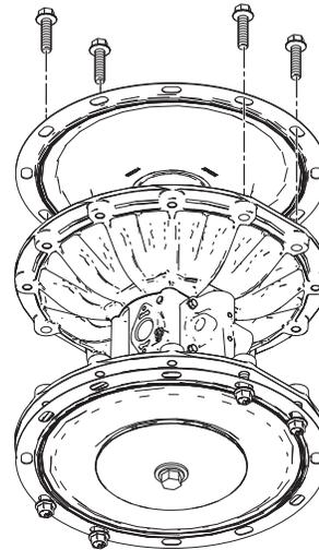
**FIG. 6. Place bolts to keep PTFE diaphragms aligned.**
