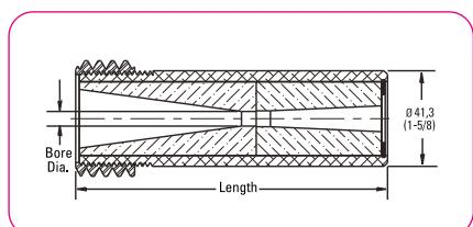
2" Thread Wide Throat Polyurethane/Aluminium Jacket Boron Carbide (Boride)
