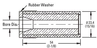
**3/4" Thread Straight Bore Boron Carbide (Boride)**
