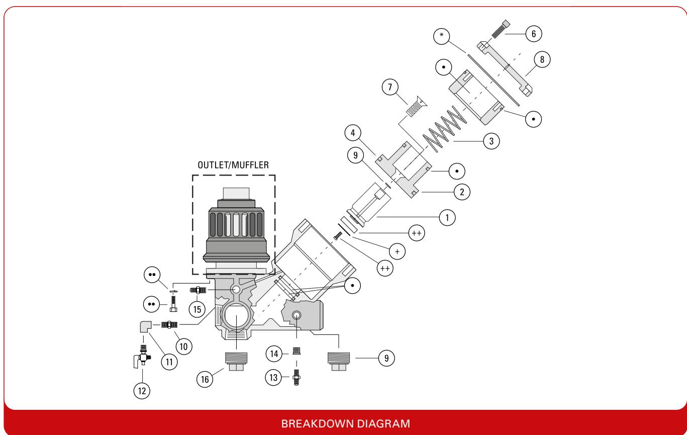
**Control Valves Inlet / Exhaust**
