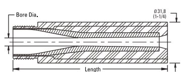
**3/4" Thread Venturi Bore Tungsten Carbide (Boride)**
