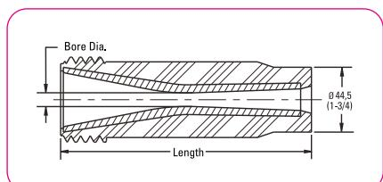
2" Thread Wide Throat Light Weight Polyurethane Jacket Ceramic Composite Liner (Boride)
