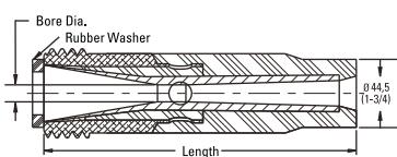
2" Coarse Thread Blast Nozzles
