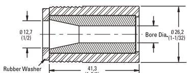
**3/4" Thread Straight Bore Tungsten Carbide (Boride)**
