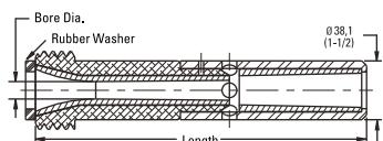
**2" Thread Double Venturi Tungsten Carbide (Boride)**
