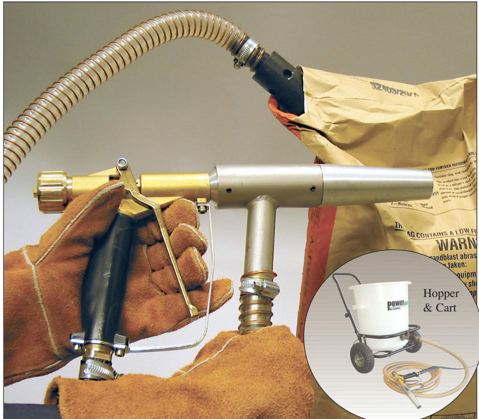
to the gun. The vacuum draws abrasive through the hose into the gun, where it mixes with compressed air. The air-abrasive mix exits the gun and strikes the surface to be blasted.
