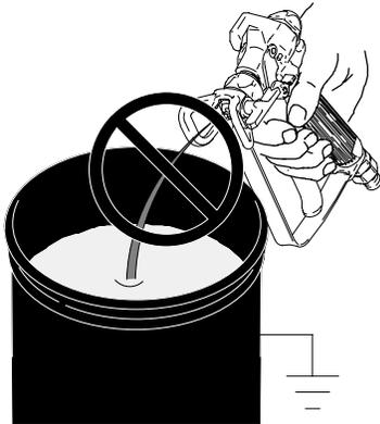
9. Try to trigger gun. No fluid should flow.
