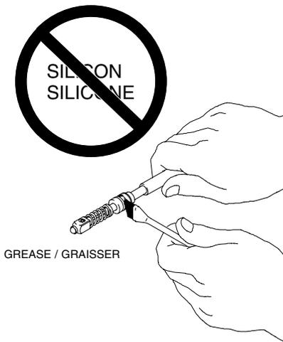
9. Grease o-rings of new needle using a *nonsilicon* grease.
