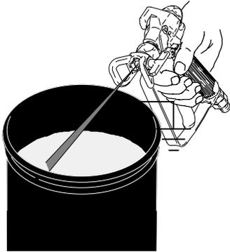
5. Trigger gun into grounded metal bucket.
