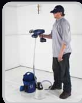
3. Turn on air compressor. Prime sprayer.
