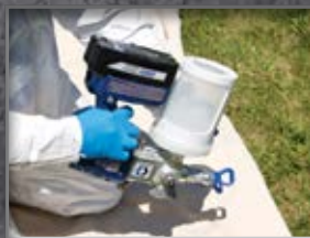
Attach cup with solvent, set to "Clean" and run upside down.
